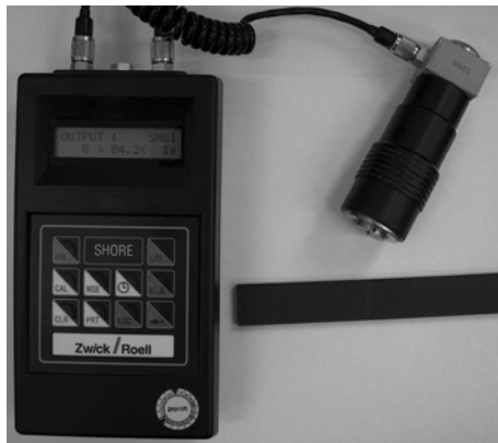
Figure 1. Shore-D hardness durometer
